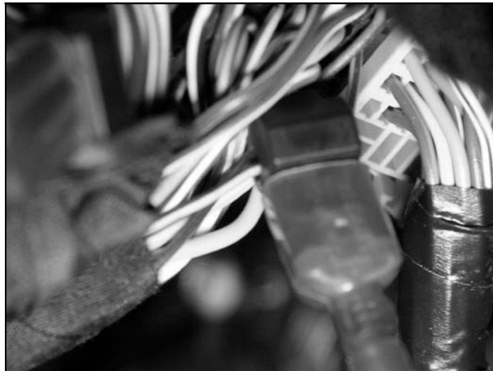
Route harness 250-8656 through the grommet in the floor board on the driver side of the truck.
