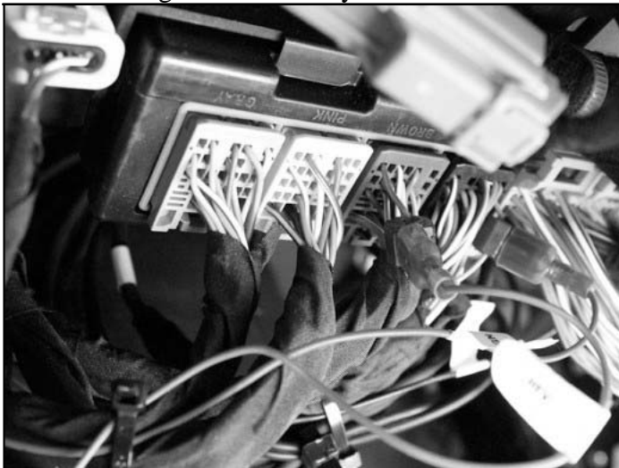
Route harness 250-8656 to the front driver side of the truck attaching it to the factory harness with cable ties.
