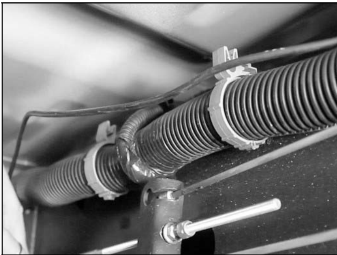
Route harness 250-8656 to the front driver side of the truck attaching it to the factory harness with cable ties.
